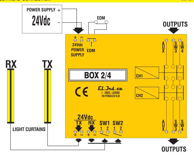
**N.B.** The unit "BOX2/4" is provide with the EDM function temporarily disabled (jumper on terminal EDM). If it becomes necessary to use other external devices (relays, etc...) to increase the output contacts, it is recommended to control the safety of these devices by remove the jumper in the terminal EDM and connect the contact or contacts NC of such devices in series in the terminal EDM.
